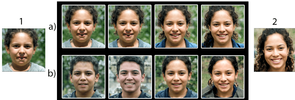
Figure 3.6: The problem of entanglement. From image 1, an interpolation is made to image 2. a) interpolation without the problem of entanglement. b) interpolation with the problem of entanglement. As can be seen, interpolation a) is much smoother and more coherent.
