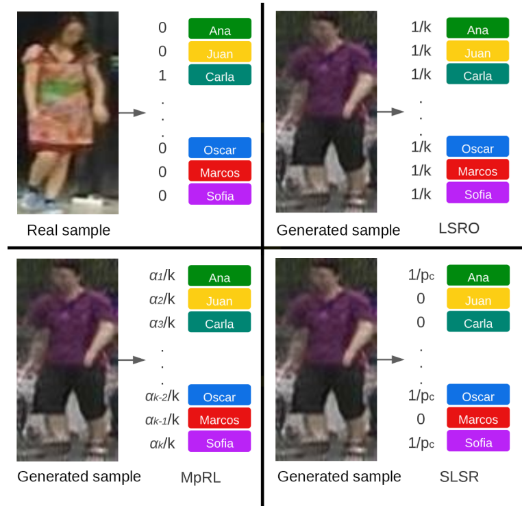
Figure 2.11: Different types of labeling. Top left: labeling of a real image corresponding to a person. LSRO: proportional labeling, k = number of classes. MpRL: labeling based on similarity. SLSR: proportional labeling based on the group to which the person belongs, p_c = distribution in the classes of the group to which they belong.
